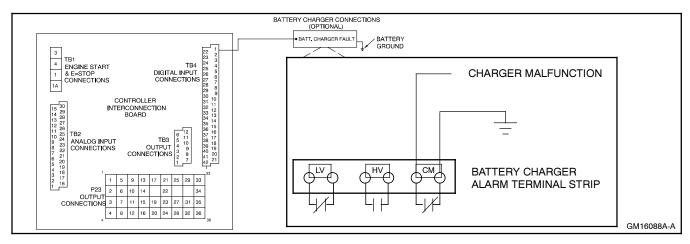
Figure 6-7 Float/Equalize Battery Charger Connections
